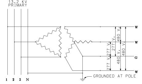
$\mathbf{G} = 0$  Volts to ground  $\mathbf{w}$  W = 277 Volts to ground
